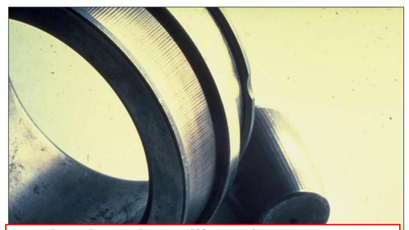
Look at the rolling elements to differentiate between vibration or electric current damages
