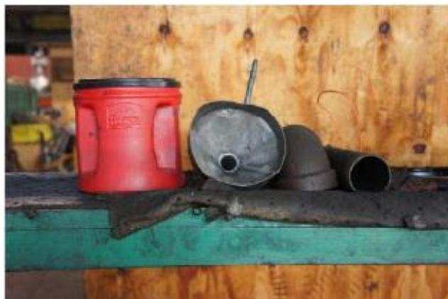
**Inadequate lubrication tools**
