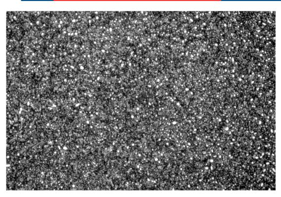
The heat treated structure must show carbides with a roundish shape and evenly distributed (= no concentation).
