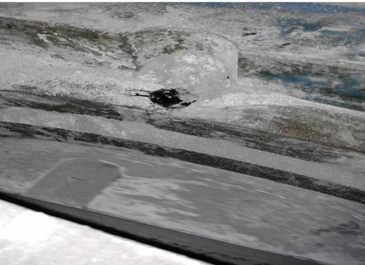
Instead of grease fitting, there is a bolt. It is clearly visible that there is a pile of dust covering the bolt. Once unscrewed, nothing stops dust to contaminate the grease
