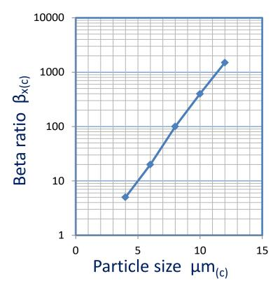
When a filter supplier talks about the micron size rating of their filter, they generally mean the micron size at which  $\beta x_{(c)} \ge 200$ .
