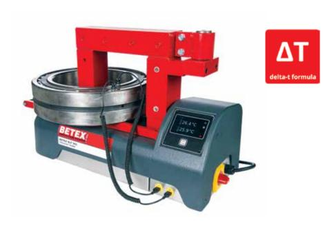
— Bearings should never be heated over 120°C (248°F), unless specified otherwise. Extreme heat can affect metallurgical structure and lubrication. Betex® Induction heaters offer full control including Delta T. When using this option, the temperature between inner- and outer ring can never exceed the maximum pre-set temperature difference.
