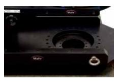
— The CRD350 Compact Ring Drive from Nexen in the customer-specific measuring system by Mahr
