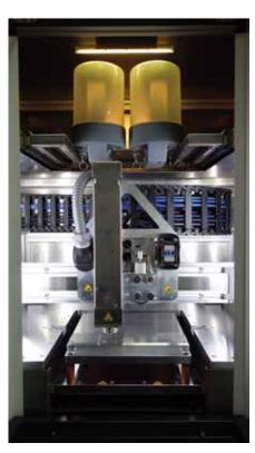
— The ExAM255 is the first industrial 3D printer worldwide producing metal pieces using injection moulding granules.
