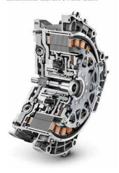
Integrated hybrid module P2. Figure courtesy of Schaeffler
