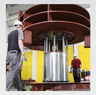
Installation of a large housing with assembled spherical plain bearing for an offshore platform
