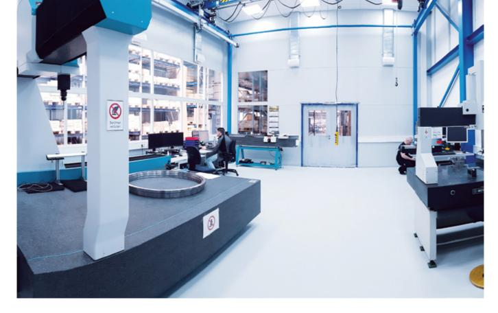
The measuring room allows Rodriguez to test the required tolerances of precision bearings and linear technology at μ.
