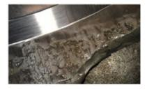
This critical bearing rotating at 24rpm was found to have failed during an ultrasound inspection. The bearing had recently been replaced, so it was relatively new. Unfortunately, the replacement bearing was not quite the correct one and was undersized for the load requirement. Very quickly, the new bearing disintegrated.
