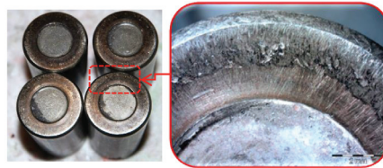
— Fig. 8 - Smearing of cylindrical roller end face
