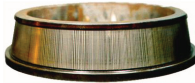
— Fig. 11 - Craters formed by current leakage resulting in fluting
