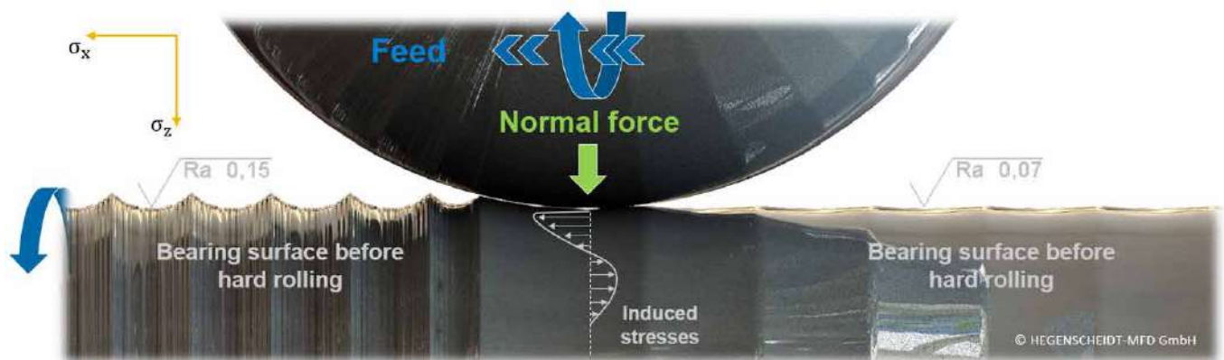
— Schematic representation of the hard rolling process
