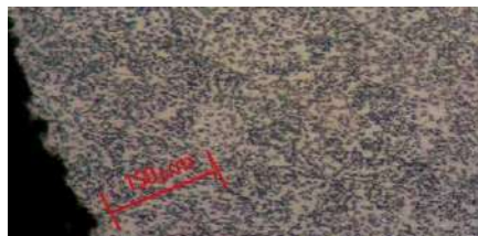
— Fig. 4: Surface depletion of carbon layer on high-speed forgings
