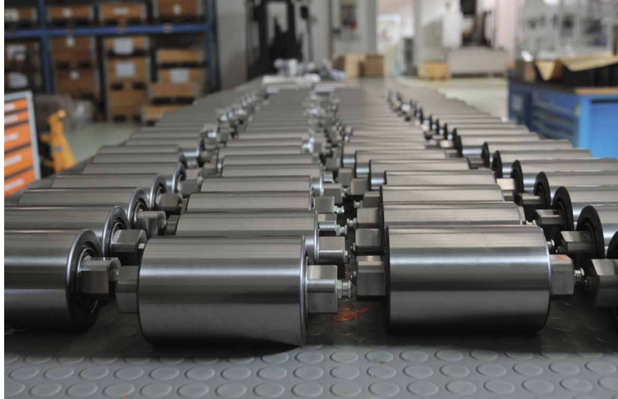
— Backup rollers tested and ready to be packed
