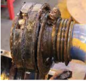
— P1: Premature bearing failure from contamination ingress
