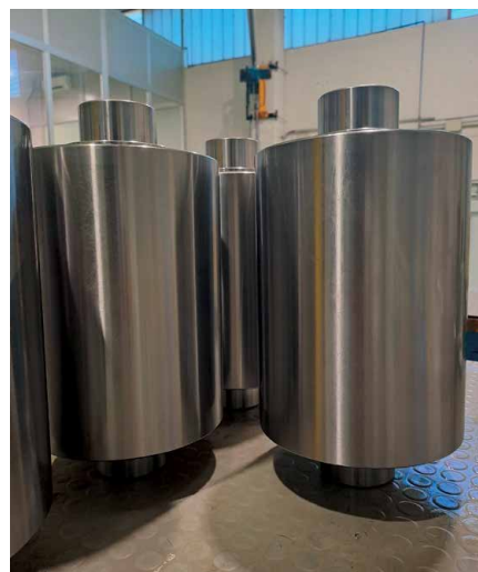
— Backup roller after revamping
