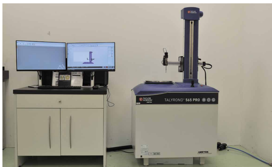
— Taylor Hobson - Ultra-high precision roundness measurement
