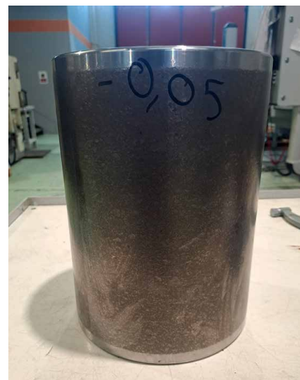
— Backup roller before revamping
