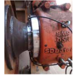
— P8: SAPO® Seal in operation
