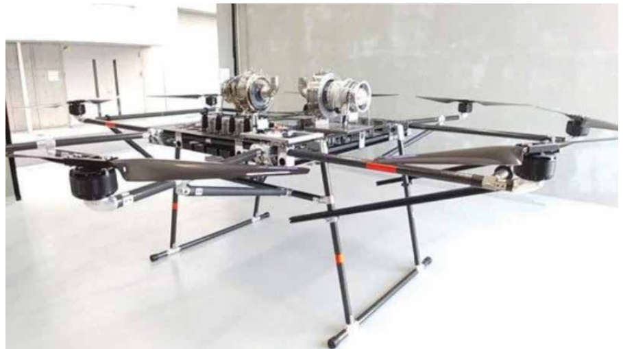
— Extending the flight range of eVTOL aircraft hinges on a variety of factors, including the high-speed revolution performance of its gas turbine generator bearings. Photo: Aero Development Japan, Inc.
