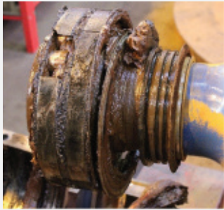
— P1: Premature bearing failure from contamination ingress
